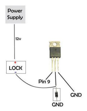
Figure 3. Connections to the Transistor TIP122.
