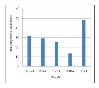
**Figure 1.** Maximum compressive load of concrete blocks made using sludge.
