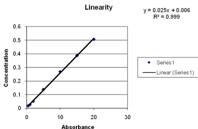
**Figure 4.** Calibration curve for Calcium Standard.
