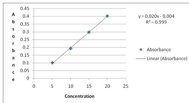
Figure 2. Calibration curve of the calcium standard.
