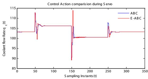
**Figure 5.** Control action comparison during servo operation.
