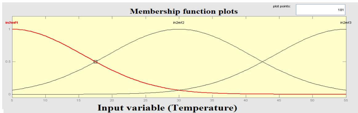
Figure 8. Temperature membership functions.
