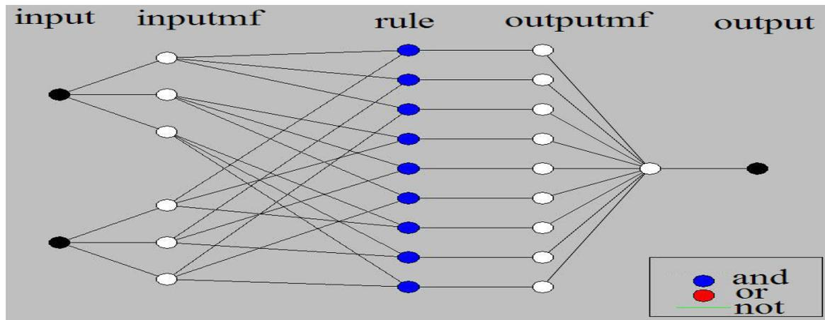
Figure 6. ANFIS controller structure.
