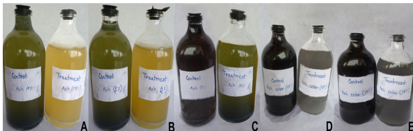
Figure 9. Effect of mixed bacterial culture on different concentrations [0.5%(A), 1%(B), 5%(C), 10%(D) and 15%(E)] of textile wastewater (acid ash color).
