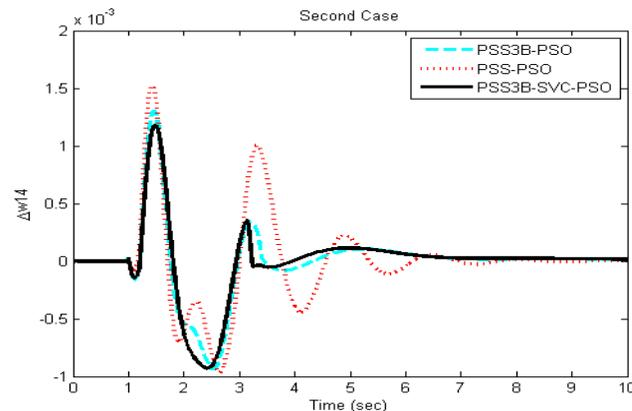
Figure 11. Inter-area mode ( $W_1-W_4$ ) of oscillation for case 2.
