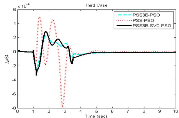
**Figure 16.** Local mode ( $W_3-W_4$ ) of oscillation for case 3.
