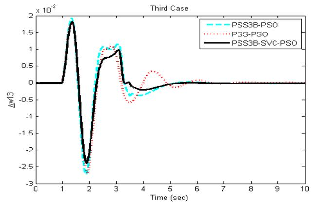
**Figure 14.** Inter-area mode ( $W_1-W_3$ ) of oscillation for case 3.
