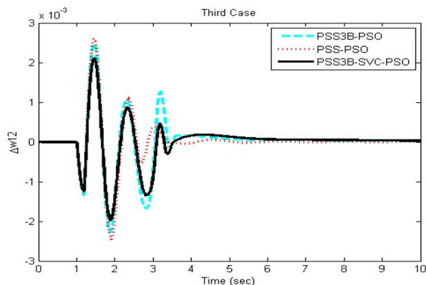
**Figure 13.** Local mode ( $W_1-W_2$ ) of oscillation for case 3.
