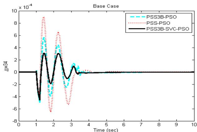
Figure 8. Local mode ( $W_3-W_4$ ) of oscillation for case 1.
