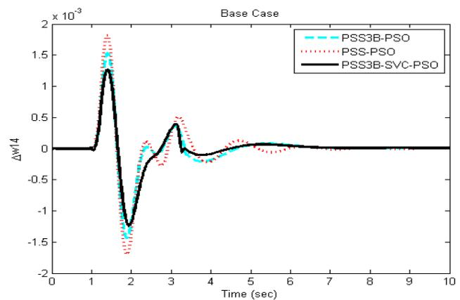
**Figure 7.** Inter-area mode ( $W_1-W_4$ ) of oscillation for case 1.
