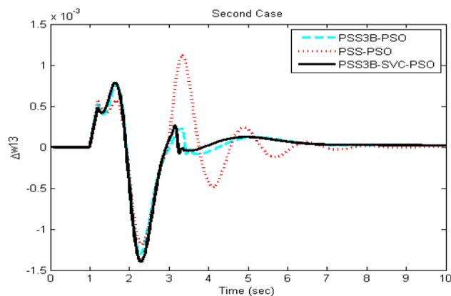
Figure 10. Inter-area mode ( $W_1-W_3$ ) of oscillation for case 2.
