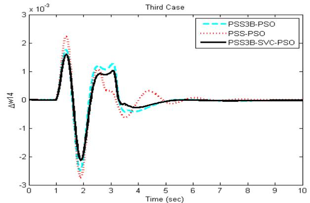
**Figure 15.** Inter-area mode ( $W_1-W_4$ ) of oscillation for case 3.
