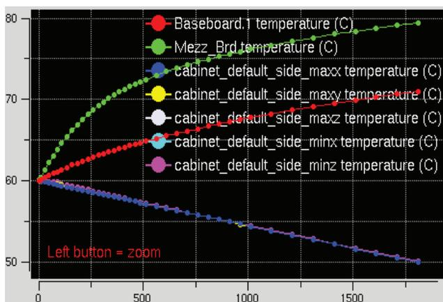
Figure 7. The temperature variation w.r.to time. (Short time operating results).
