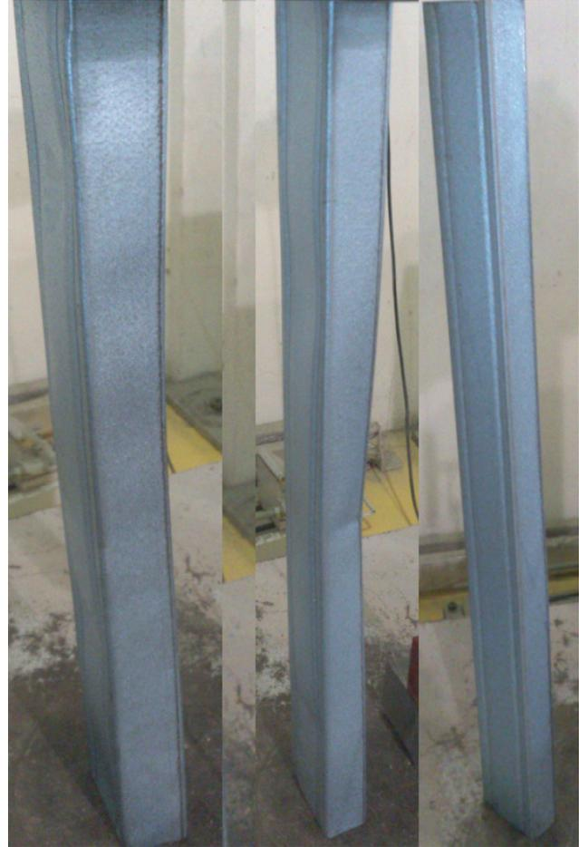
**Figure 2.** Failure modes shapes.
