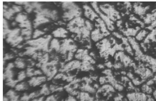
Fig. 9. Microstructure of Al 7072/SiC metal matrix composite, 200X
