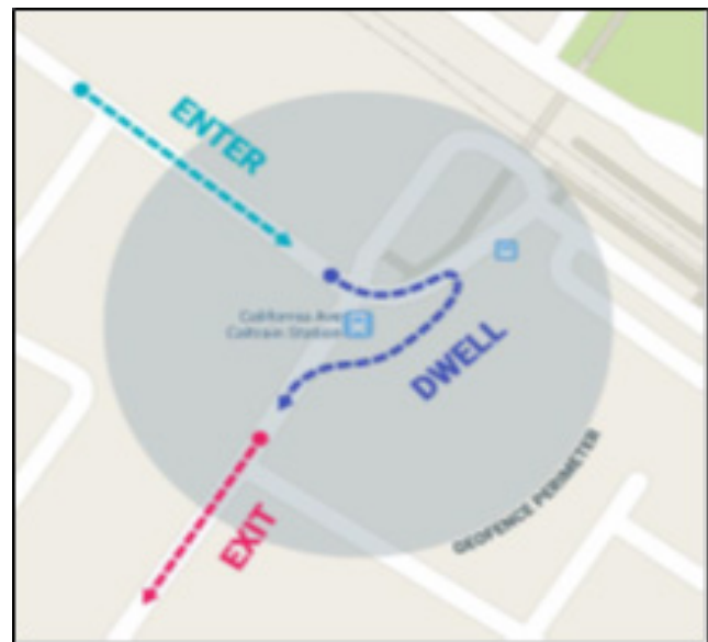
Figure 7. Basic Concept of Geo-Fencing.
