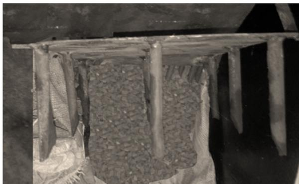
**Figure 1.** Model flexible pile raft system of 9 piles.
