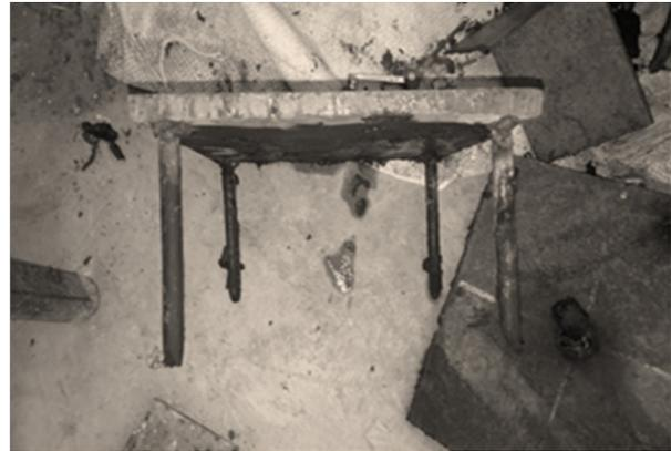
**Figure 2.** Model rigid pile raft system of 4 piles.
