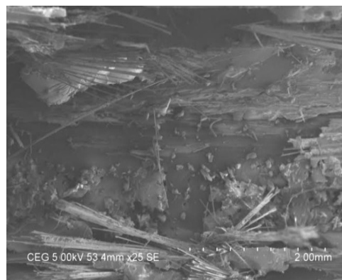
Figure 6. SEM micrograph of the composite sample subjected to impact loading.
