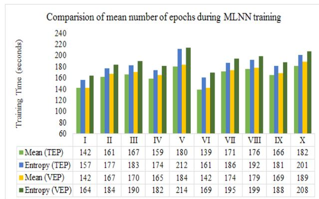
Figure 7. Comparison of mean number of epochs for the MLNN using mean and entropy features.
