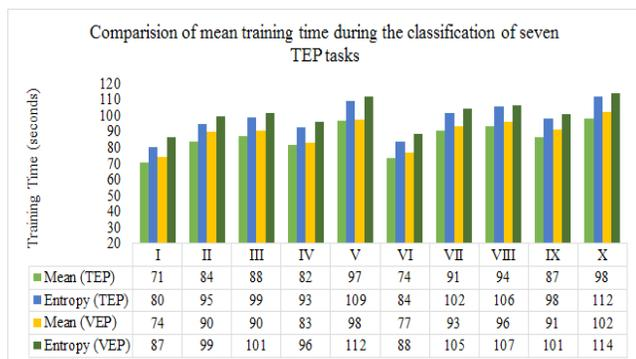
Figure 6. Comparison of mean training time for the MLNN using mean and entropy features.
