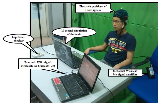
**Figure 4.** Experimental setup during the acquisition of tasks to command custom-IRCC.
