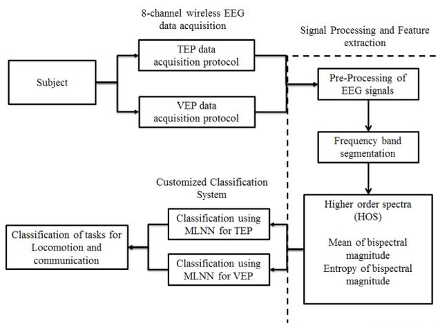
**Figure 1.** Block diagram of the proposed custom-IRCC using TEP and VEP response.
