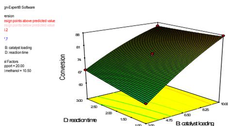
**Figure 10.** Interaction between catalyst loading and reaction time.
