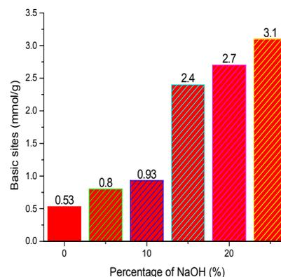
Figure 3. Basic sites of the synthesized catalysts.
