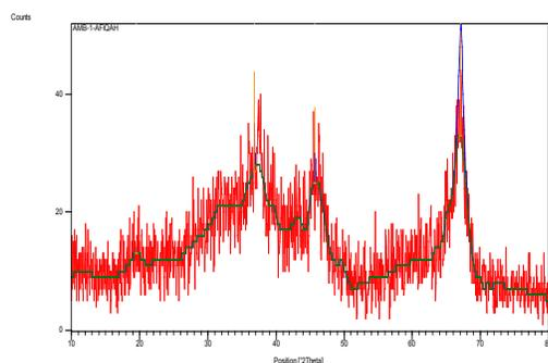
Figure 1. XRD pattern of calcined alumina bead.
