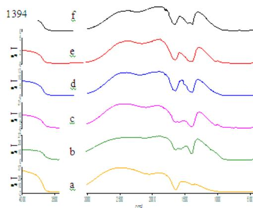
Figure 2. FTIR spectra of. (a) 0% Na/Al-beads. (b) 5% Na/Al-beads. (c) 10% Na/Al-beads. (d) 15% Na/Al-beads. (e) 20% Na/Al-beads. (f) 25% Na/Al-beads.
