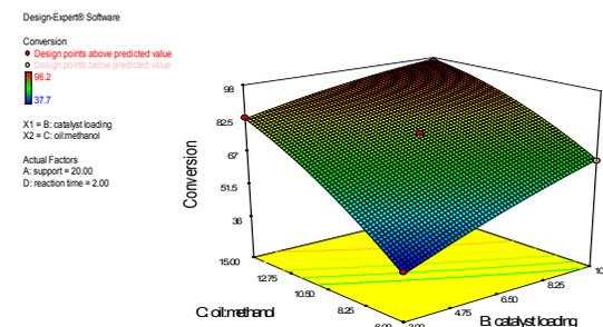
Figure 9. Interaction between catalyst loading and molar ratio.
