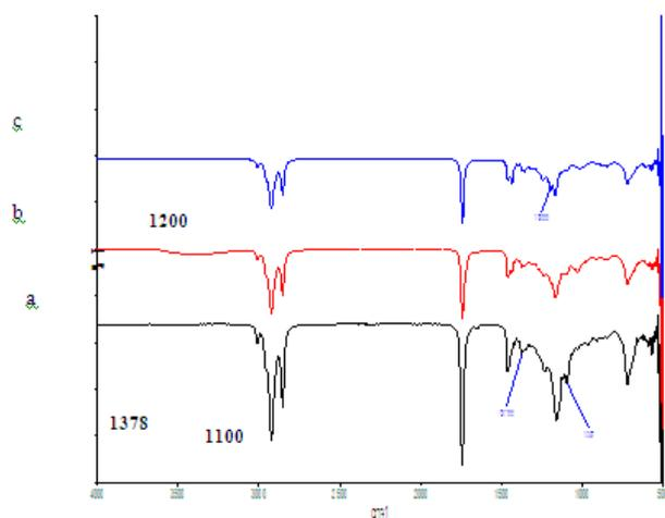
**Figure 4.** FTIR-ATR spectra of. (a) Corn oil. (b) Biodiesel from 10% Na/Al-beads. (c) Biodiesel from 15% Na/Al-beads.
