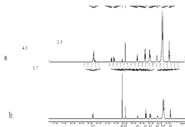
**Figure 5.** NMR spectra of biodiesel from. (a) 10% Na/Al-bead. (b) 15% Na/Al-bead.
