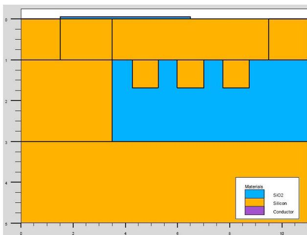
**Figure 3.** LDMOS device structure from process simulation
