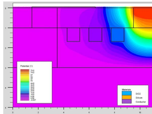
Figure 8. Electric Potential distribution under breakdown condition.
