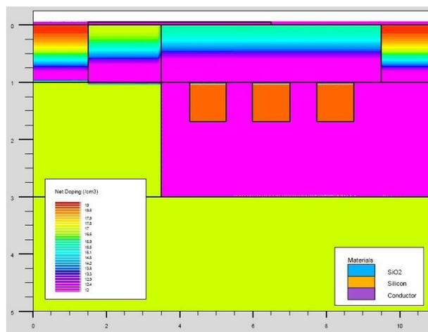
**Figure 5.** Net doping in proposed LDMOS device.
