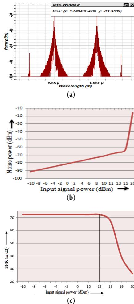
**Figure 10.** (a) Optical spectrum at the output of fiber when two wavelengths are transmitted using QAM modulation. (b) Graph between Input signal power and noise power for QAM modulation. (c) Graph between Input signal power and SNR for QAM modulation
