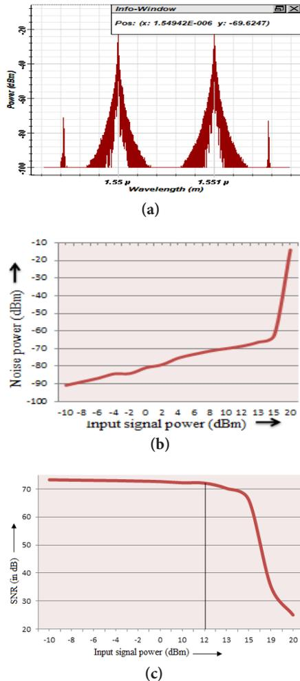
**Figure 12.** (a) Optical spectrum at the output of fiber when two wavelengths are transmitted using DPSK modulation. (b) Graph between Input signal power and noise power for DPSK modulation. (c) Graph between Input signal power and SNR for DPSK modulation
