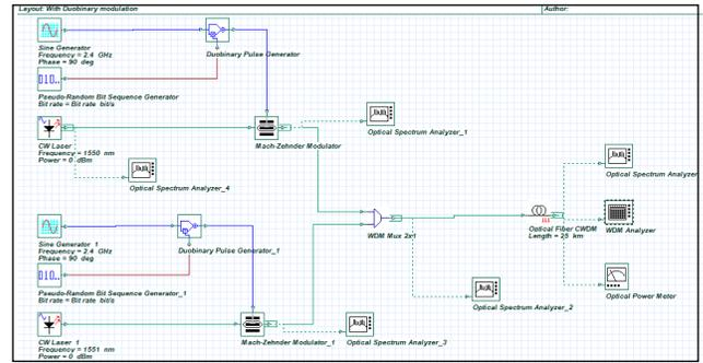
**Figure 2.** Simulation Setup for WDM PON Architecture for transmission of two input wavelengths by use of Duobinary Modulation in OptiSystem Software
