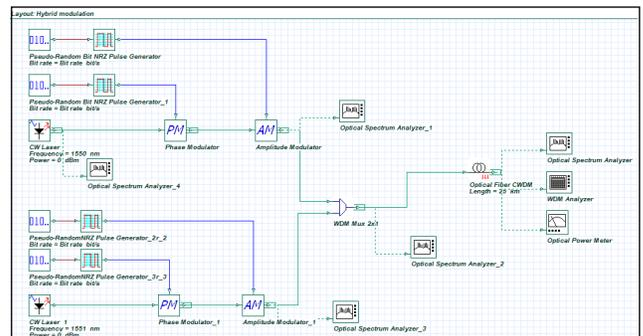
**Figure 3.** Simulation Setup for WDM PON Architecture for transmission of two input wavelengths by the use of Hybrid Modulation in OptiSystem Software
