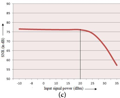
**Figure 8.** (a) Optical spectrum at the output of fiber when two wavelengths are transmitted using Duobinary modulation. (b) Graph between Input signal power and noise power for duobinary modulation. (c) Graph between Input signal power and SNR for duobinary modulation
