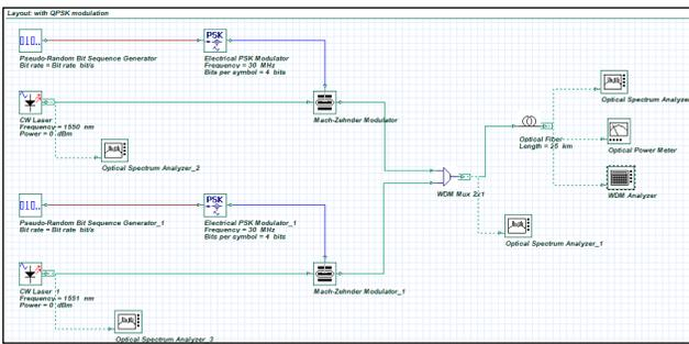
**Figure 5.** Simulation Setup for WDM PON Architecture for transmission of two input wavelengths by the use of QPSK Modulation in OptiSystem Software
