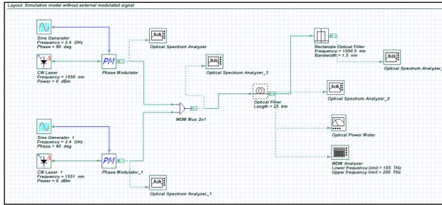
**Figure 1.** Simulation setup for WDM PON architecture for transmission of two input wavelengths by use of Filter in OptiSystem software.
