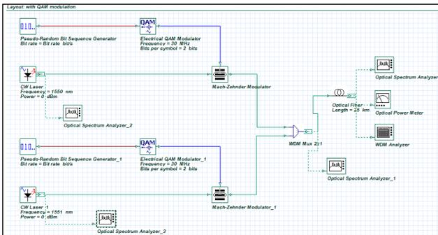
**Figure 4.** Simulation Setup for WDM PON Architecture for transmission of two input wavelengths by the use of QAM Modulation in OptiSystem Software
