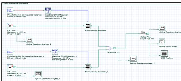
**Figure 6.** Simulation Setup for WDM PON Architecture for transmission of two input wavelengths by the use of DPSK Modulation in OptiSystem Software
