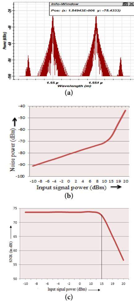
**Figure 9.** (a) Optical spectrum at the output of fiber when two wavelengths are transmitted using Hybrid modulation. (b) Graph between Input signal power and noise power for hybrid modulation. (c) Graph between Input signal power and SNR for hybrid modulation
