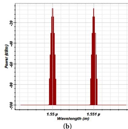
**Figure 7.** (a) Optical spectrum at the output of fiber when two wavelengths are transmitted without any external modulation. (b) Optical spectrum at the output of filter when two wavelengths are transmitted without any external modulation
