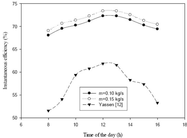
**Figure 5.** Variation of instantaneous collector efficiency with respect to time.
