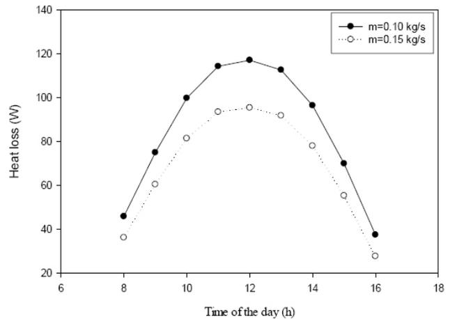
**Figure 7.** Variation heat loss with respect to time.
