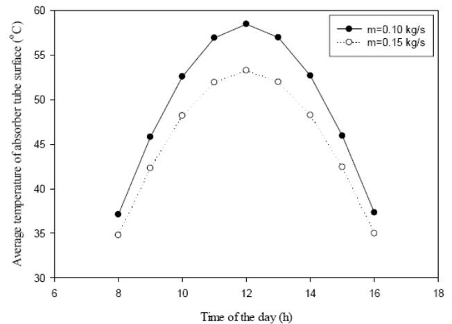
**Figure 4.** Variation of average temperature of absorber tube surface with respect to time.
