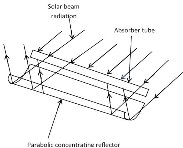
**Figure 1.** Schematic view of a parabolic concentrating reflector.
