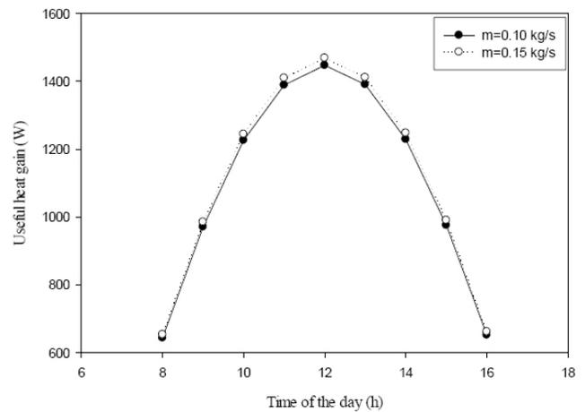
**Figure 3.** Variation of useful heat gain with respect to time.
