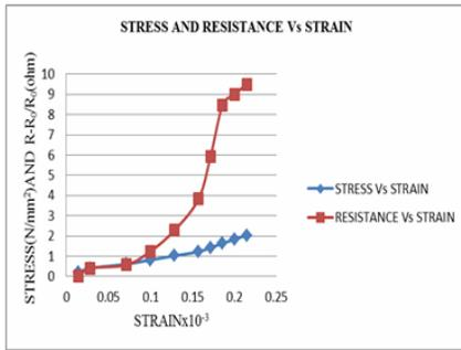
Figure 6. Carbon fibre, methyl cellulose and silica fume (along stress axis).
