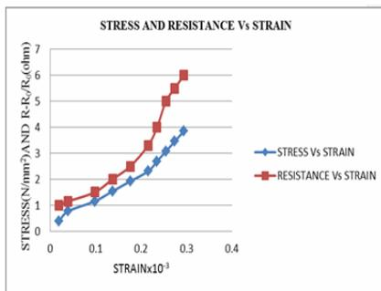
Figure 7. Carbon fibre, methyl cellulose and silica fume (perpendicular to stress axis).
