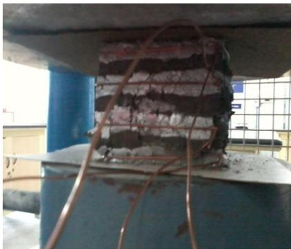
Figure 3. Cube-compressive failure.
