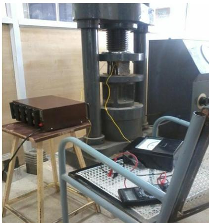
Figure 2. Four probe method.
