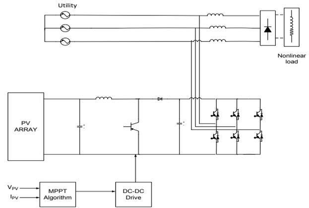
Figure 1. PV-active power filter system configuration.
