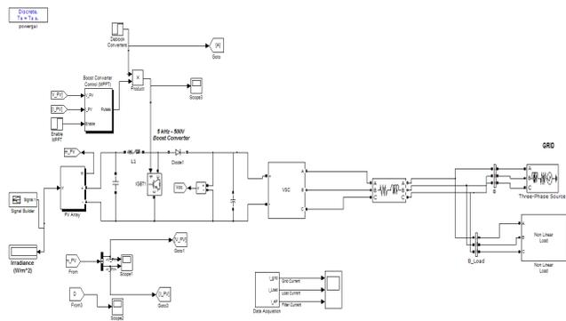
Figure 7. MATLAB design of PV-APF system with PI controller.
