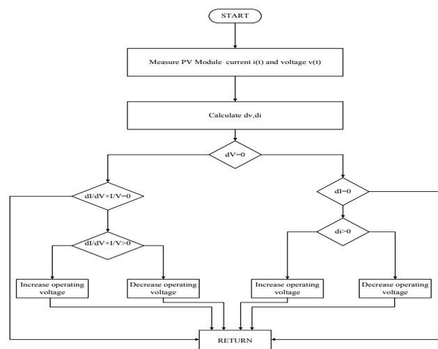
**Figure 4.** INC mechanism flow chart.
