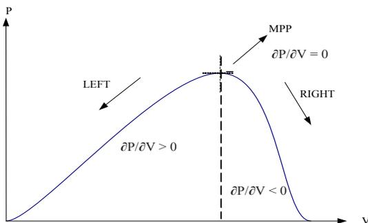
**Figure 3.** PV power curve specifying fundamental ideology of incremental conductance.
