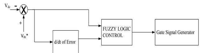
Figure 5. Fuzzy logic control scheme.
