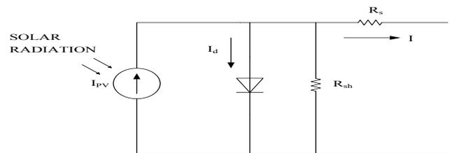
Figure 2. Diagrammatical representation of PV module.
