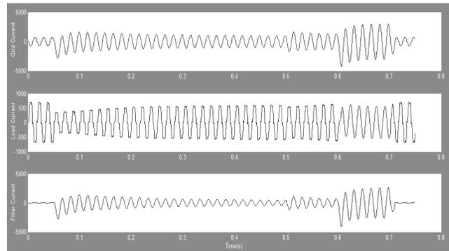
Figure 8. Simulation results for APF with PI Controller (a) Grid current. (b) Load current. (c) Filter current.
