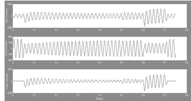
Figure 10. Simulation results for APF with Fuzzy Controller (a) Grid current. (b) Load current. (c) Filter current.
