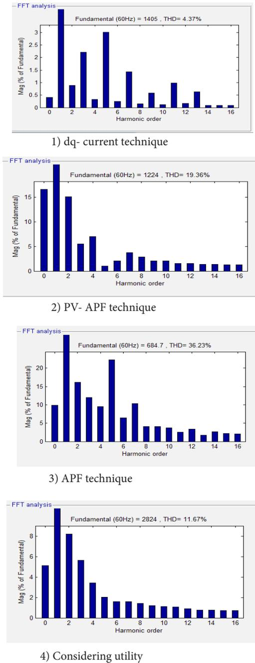
Figure 9. FFT analysis of grid current in various modes with PI controller.
