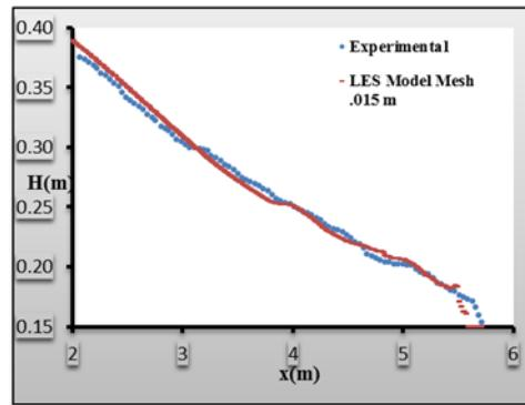
**Figuer 7.** Water free surface profiles in LES turbulence model and the experimental results ( $t = 1.25$  s)
