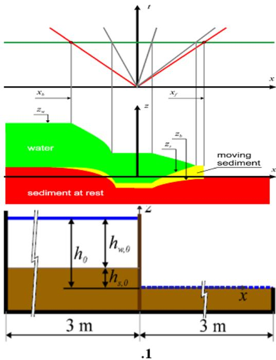
**Figure 1.** Schematic figure of the dam break on the mobile bed (left)33, profile of positive wave caused by dam failure with measured variables (right)17
