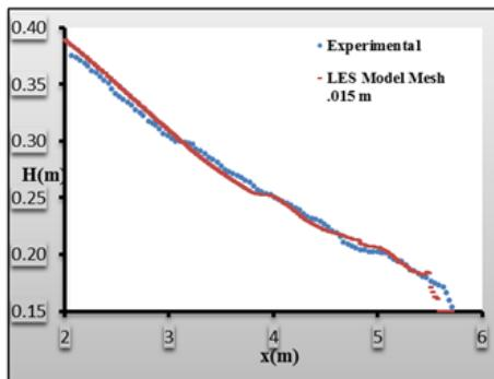
**Figuer 9.** Water free surface profiles in LES turbulence model and the experimental results ( $t = 1.25$  s)
