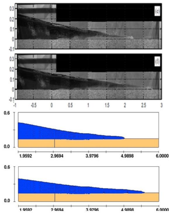
**Figuer 3.** The movement of positive wave after pulling the valve in time  $t = 1, 1.25$  seconds in the experimental model (left) and in the Flow-3D (right), the results of the simulation by LES turbulence modelturbulence model
