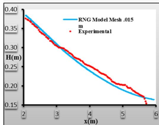
**Figuer 4.** Water free surface profiles in models of Prandtl mixing length, turbulence kinetic energy,  $k-\epsilon$  and RNG ( $t = 1.25$  s)modelturbulence model
