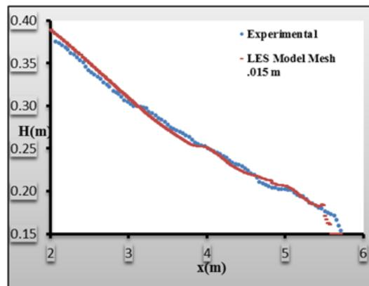
**Figuer 5.** Water free surface profiles in LES turbulence model and the experimental results ( $t = 1.25$  s)
