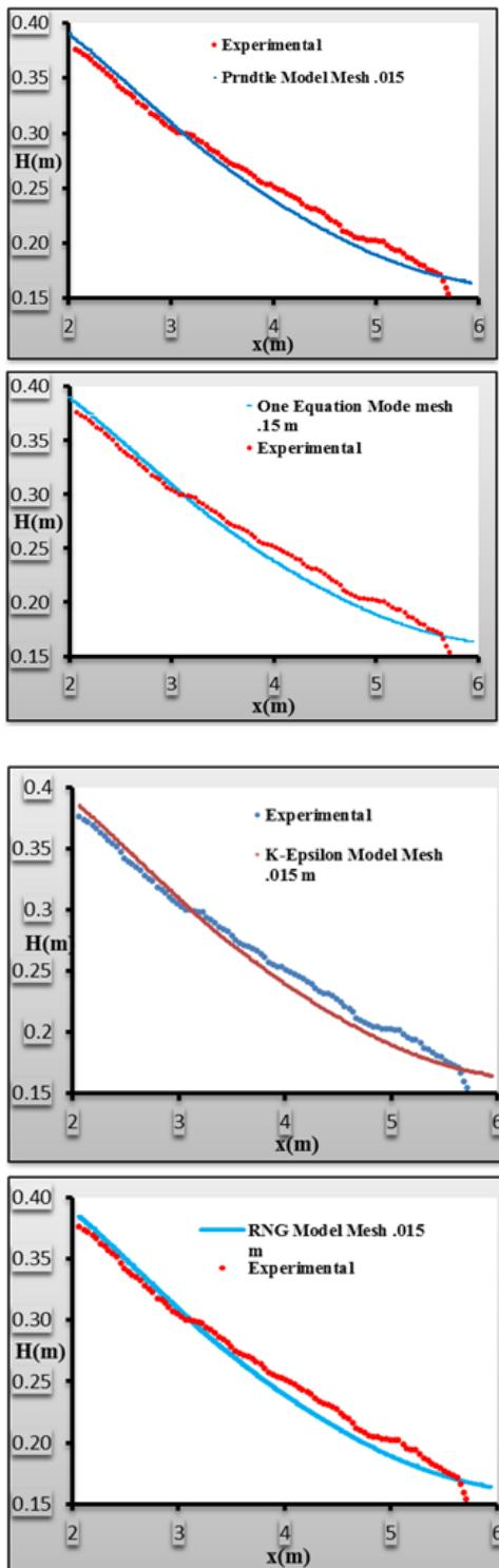
**Figuer 6.** Water free surface profiles in models of Prandtl mixing length, turbulence kinetic energy, k- $\epsilon$  and RNG ( $t = 1.25$  s)
