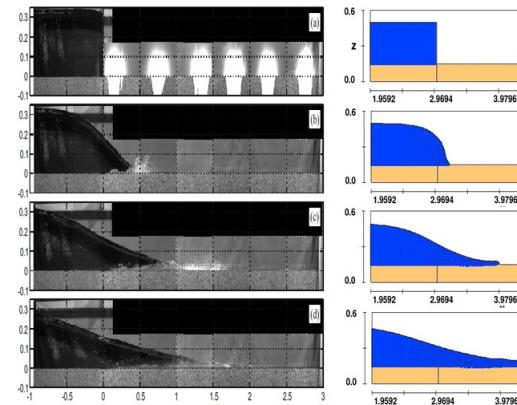
**Figure 2.** Formation and motion of the positive wave after pulling the valve in time  $t = 0, 0.25, 0.5, 0.75$  second in the experimental model (left) and in the Flow-3D (right), the results of the simulation by LES turbulence model
