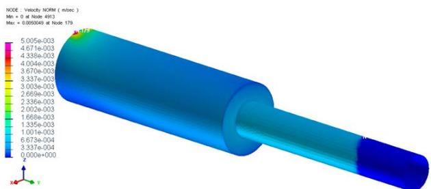
**Figure 7.** Distribution of resin velocities throughout volume of preform model of nominal size 100×40×20 mm in case of point-feeding of resin (time t=96,01 s).
