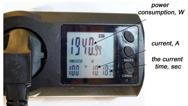
Figure 2. ROBITON PM-2 power meter display
