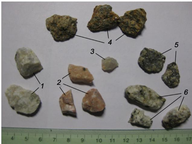
**Figure 10.** Grains of Crushed Granite Stone Sized 10-20 mm (One Sample Material): 1 – Plagioclase Grains; 2 – Microcline Grains; 3 – Quartz Grain; 4 – Grains with Sign of Weathering; 5 – Grains Containing Intergrown Plagioclase, Amphibole and Biotite; 6 – Grains, Containing Intergrown Plagioclase and Amphibole.
