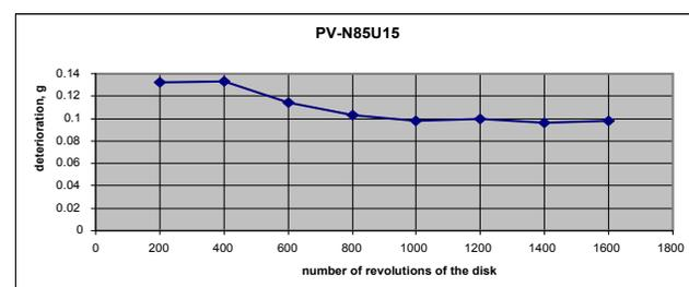
**Figure 4.** Abrasive wear curve for IIB-H85IO15 powder coating.
