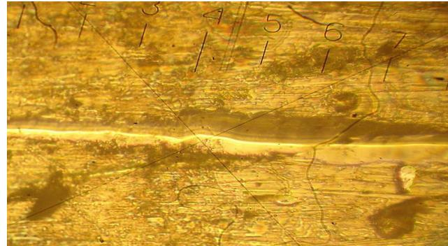
**Figure 5.** Footprints of diamond indenter in the transitory zone on the surface of detonation-coated specimen.
