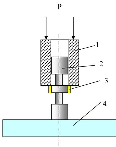
**Figure 3.** Coatings. Shear test configuration. 1. Liner, 2. Specimen, 3. Coating on the specimen, 4. Bench. P load on liner is shown using arrows. Inner liner diameter: 18 mm, belt diameter (under coating 3): 17.8 mm.
