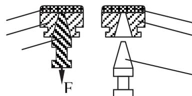
**Figure 1.** Measuring adhesion: 1. Taper pin, 2. Taper hole liner, 3. Coating.
