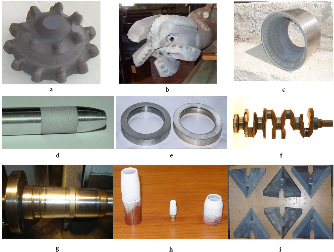
**Figure 6.** Applications of detonation coatings.
