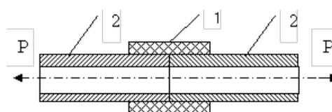
**Figure 2.** Measuring cohesion: 1. Coating, 2. Steel tube, P. Tensile strength.
