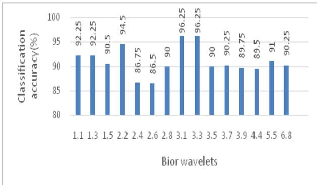
Figure 6. Classification accuracy of Bior wavelets.
