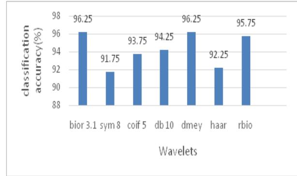
Figure 8. Classification accuracy of wavelets.
