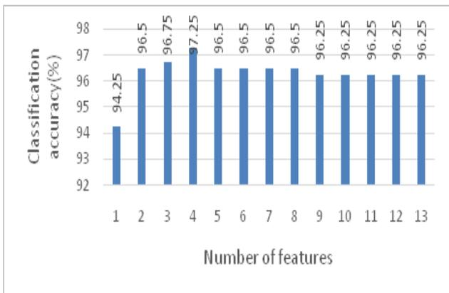
Figure 10. Effect on classification accuracy with number of features.
