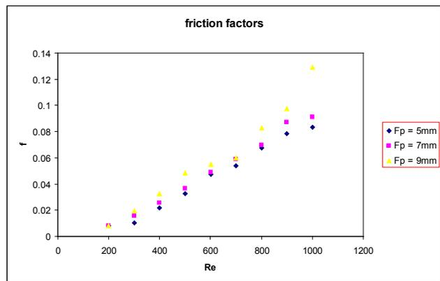
Figure 3. The comparison of f factors of various fin pitches for laminar.
