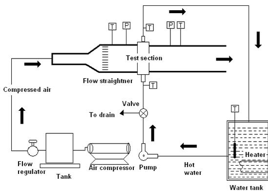
Figure 2. Schematic of experimental setup.
