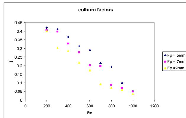
Figure 4. The comparison of j factors of various fin pitches for laminar.
