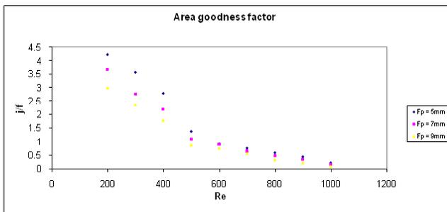
Figure 7. Comparison of  $j/f$  values of various fin pitches for laminar.
