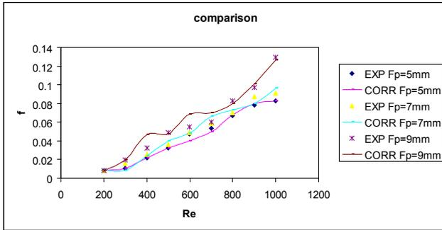
Figure 5. Comparison of  $f$  experimental results with correlation (laminar).
