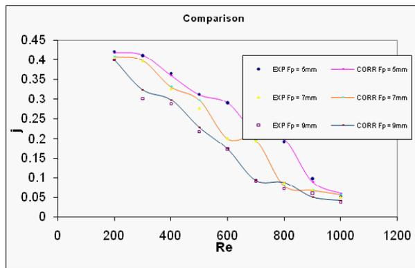
Figure 6. Comparison of  $j$  experimental results with correlation (laminar).
