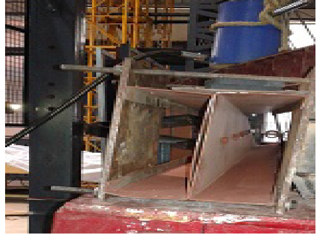
Figure 11. Experimental arrangement of 230 mm depth beam for torsional.
