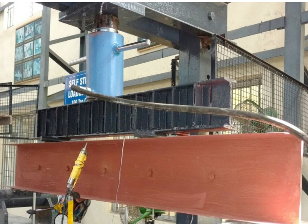
Figure 9. Experimental arrangement of 230 mm depth beam for flexural.
