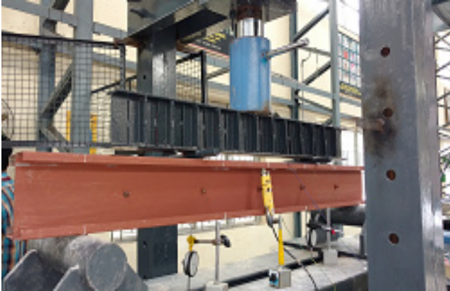
Figure 8. Experimental arrangement of 180 mm depth beam for flexural.
