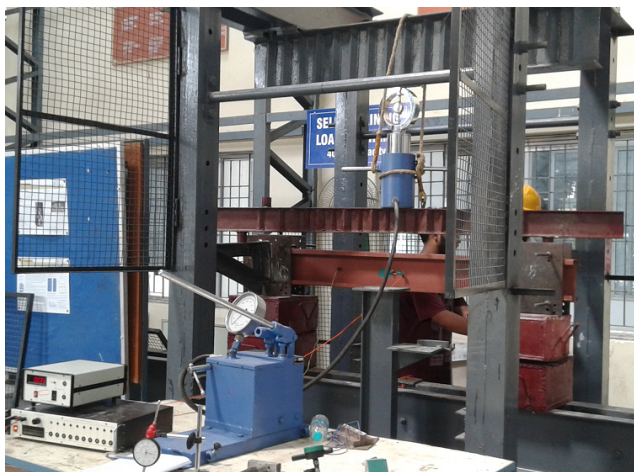
Figure 10. Experimental arrangement of 180 mm depth beam for torsional.
