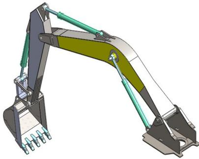
Figure 1. 30-Ton excavator (design model)
