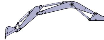
Figure 2. Max. digging radius position.
