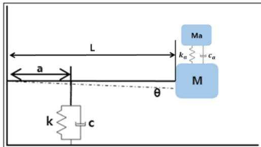
Figure 5. Tuned mass damper model.
