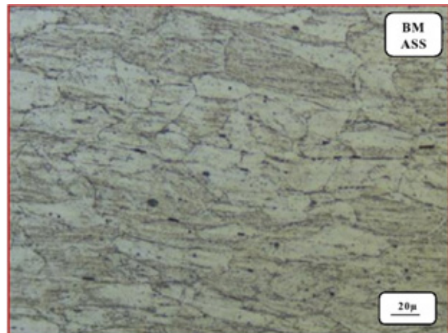
Figure 7. BM ASS microstructure.
