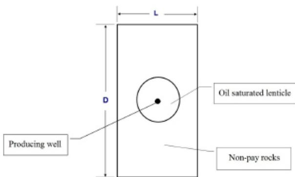
**Figure 9.** Schematic layout of the well location in the development of the lenticle placed in low permeability reservoir. L=10 km, D=20 km.
