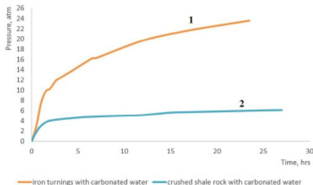
**Figure 5.** Pressure dynamics in the experiments with iron turnings and crushed shale rock.
