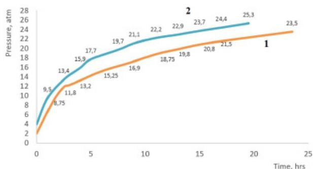
**Figure 3.** Dynamics of reactor pressure during stationary experiments with initial pressure values of (1) 2 atm and (2) 4 atm.
