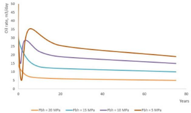
**Figure 10.** Dynamics of oil production rate during lenticle development under depletion drive.
