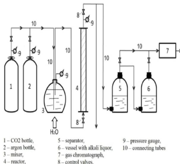
**Figure 2.** Schematic layout of laboratory plant for dynamic experiments.
