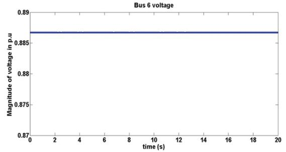
Figure 12. Bus 6 voltage with STATCOM.
