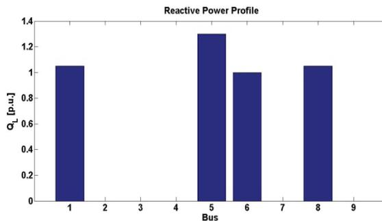
Figure 8. Reactive power (load) without STATCOM.
