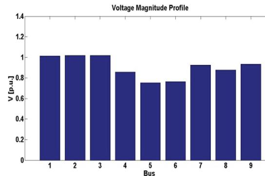
**Figure 2.** Voltage profiles without STATCOM.
