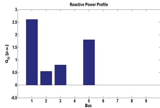
Figure 14. Reactive Power (generator) with STATCOM.
