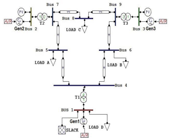
Figure 1. WSCC 9 bus in power system.
