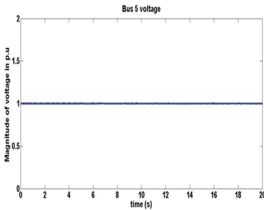
Figure 11. Bus 5 Voltage with STATCOM.
