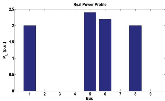
Figure 7. Real power (load) without STATCOM.
