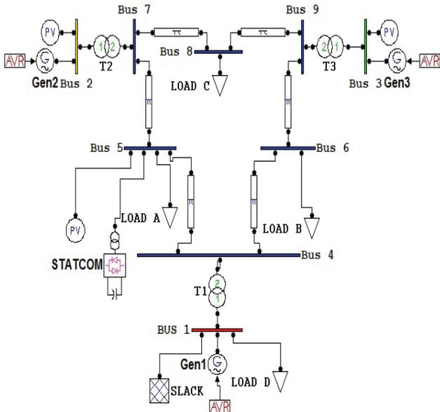
Figure 9. WSCC 9 bus system with STATCOM.
