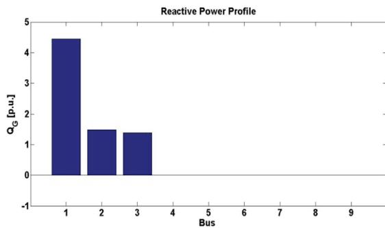
Figure 6. Reactive power (generator) without STATCOM.
