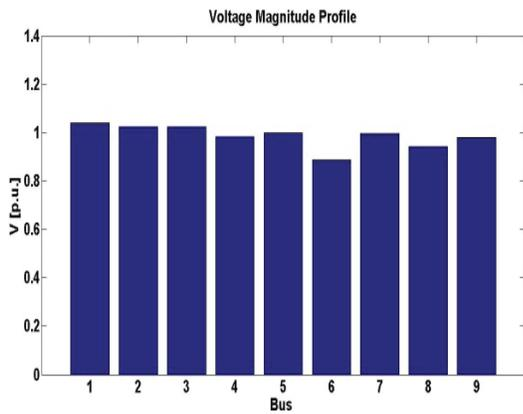
Figure 10. Voltage profile with STATCOM
