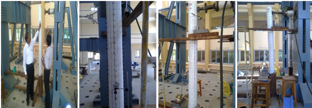
Figure 3. CLateral Load Test on Conventional RCC Pile Elements at Free End.
