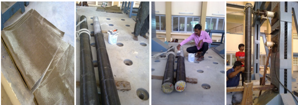
Figure 4. BFRP Wrapping in Hoop Directional (0° orientation) and Retrofitted RCC Pile Elements Test.
