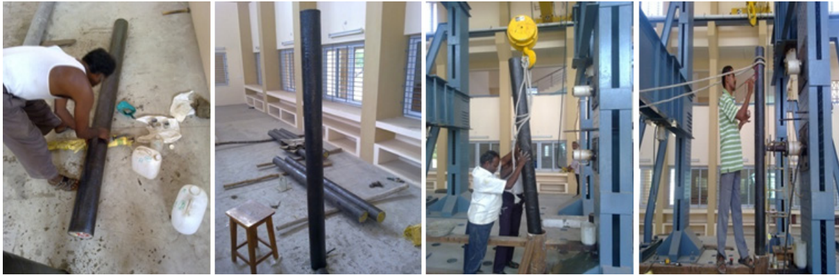
Figure 5. BFRP Wrapping in Vertical Direction ( 90^\circ orientation) and Retrofitted RCC Pile Elements Test.
