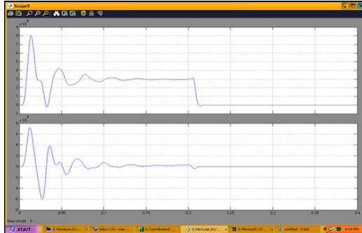
**Figure 22.** Real (top) and reactive (bottom) power dispatched by the grid.
