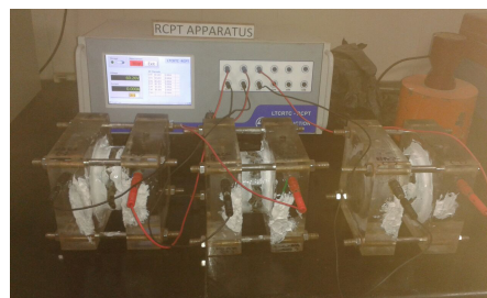
Figure 12. Rapid chloride penetration test
