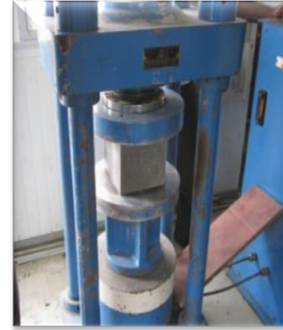
Figure 11. Compressive strength testing.
