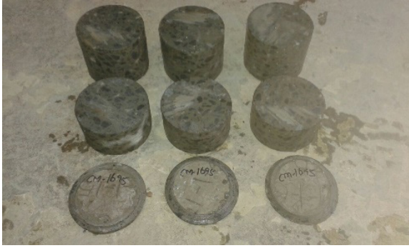
Figure 9. Core cut specimen for RCPT.
