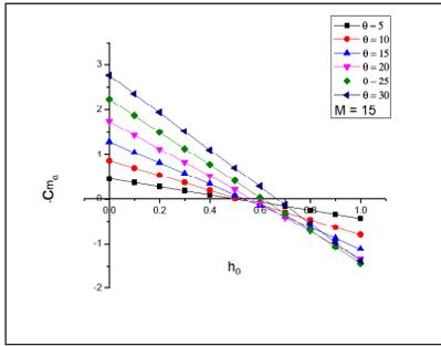
**Figure 7.** Variation of stiffness derivative for M=15 with pivot position.
