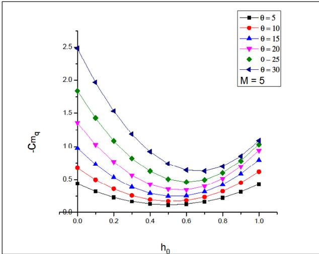
**Figure 2.** Variation of damping derivative for M=5, with pivot position.
