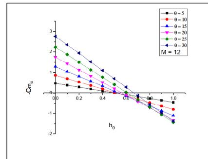
**Figure 5.** Variation of stiffness derivative for M=12 with pivot position
