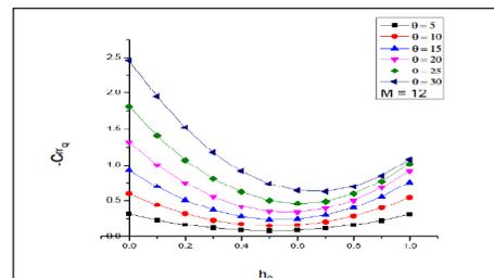
**Figure 6.** Variation of damping derivative for M=12 with pivot position.
