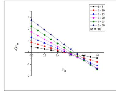
**Figure 3.** Variation of stiffness derivative M=10 with pivot position.
