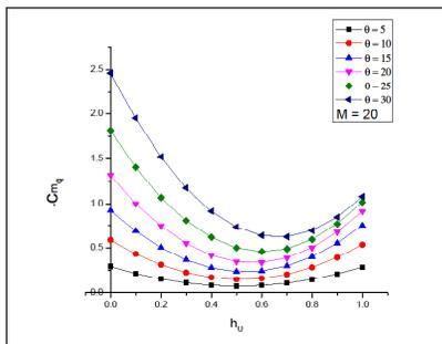
**Figure 10.** Variation of damping derivative for M=20 with pivot position.
