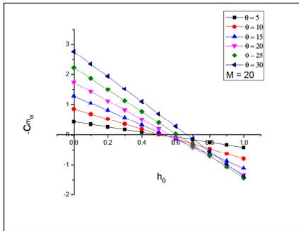
**Figure 9.** Variation of stiffness derivative for M=20 with pivot position.
