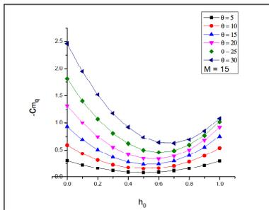
**Figure 8.** Variation of damping derivative for M=15 with pivot position.
