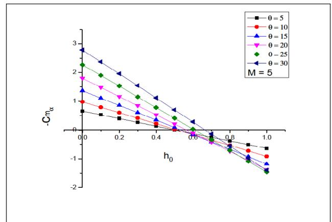
Figure 1. Variation of Stiffness derivative for M=5 with pivot position.
