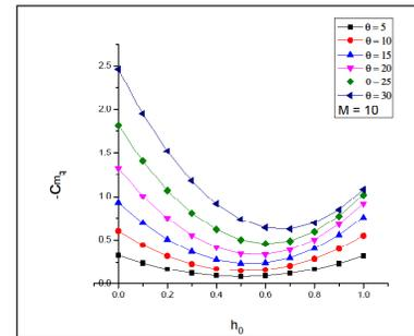
**Figure 4.** Variation of damping derivative for M=10 with pivot position.
