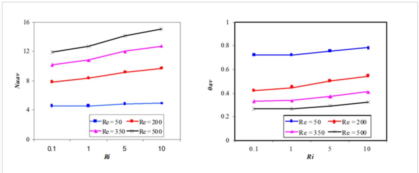
Figure 6 illustrates average Nusselt number at the heated wall and bulk average fluid temperature in the cavity for different values of  $Re$ . It is seen that for low Reynolds number heat transfer rate at the bottom wall is about stationary with respect to  $Ri$  and maximum heat transfer is found for the largest value of  $Re$  which is reasonable. A reverse effect is followed for the case of average temperature of the fluid inside the cavity.
