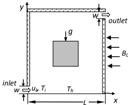
For a steady state, two-dimensional, laminar, incompressible flow of a Newtonian and electrically conducting fluid with constant thermophysical properties, the governing differential equations designed for the present problem in the dimensionless form consisting of the conservation of mass, momentum, and energy can be expressed as
