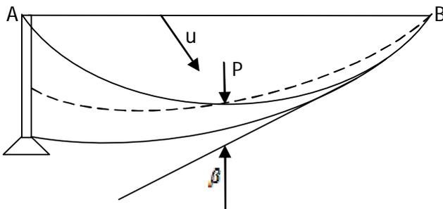
Fig. 3: Shows the beam at the second equilibrium state. The beam bends laterally as well as twists. The fibres at the middle of the beam may also warp.
