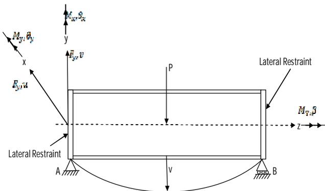
Fig. 1: Shows vertical bending of an I-beam with end restraints against lateral buckling. This bending represents the first equilibrium state of beam.
