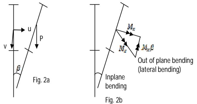
Fig. 2a: Shows section of the beam at the second equilibrium state. The beam bends laterally as well as twists. Fig. 2b: Shows contribution of vertical bending
