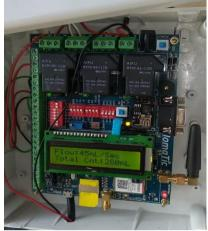
Fig 5: Water Supply Counting Display
