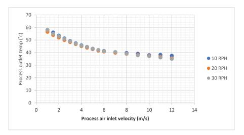
Figure 5. Changes Process Outlet Temperature with Process Inlet Air Velocity for Different Rotational Speed.
