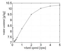
Figure 3: Air outlet water content for different desiccant wheel rotating speeds
