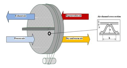
Figure 1: Schematics of a desiccant wheel
