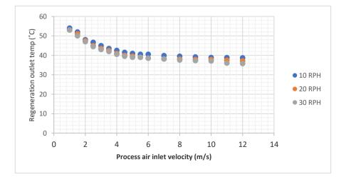
Figure 7. Changes in Reactivation Outlet Temperature with Process Inlet Air Velocity for Different Rotational Speed
