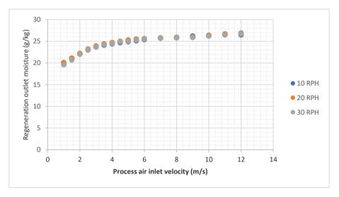
Figure 6. Changes in Reactivation Outlet Moisture with Process Inlet Air Velocity for Different Rotational Speed
