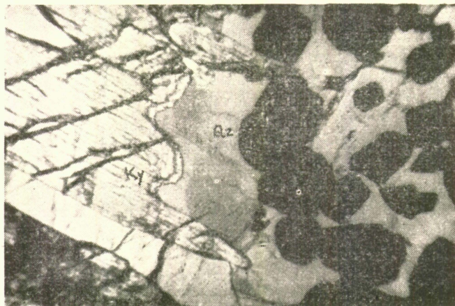
Figure 1. Cavity-filling kyanite being replaced by quartz. The latter enclosing ore minerals (ilmenite and magnetite), in polarised light \times 90 .
