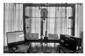
Fig. 1: Experimental setup for testing MR damper
