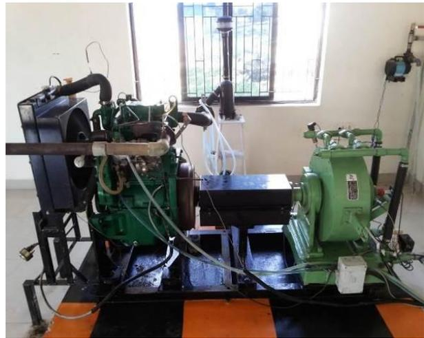
Fig. 1: Naturally aspirated engine setup
