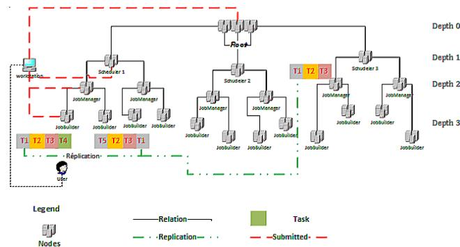
Figure 3. CLOAK-Reduce Architecture
