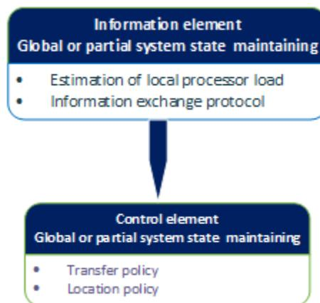
Figure 2. Structure of a dynamic allocation algorithm
