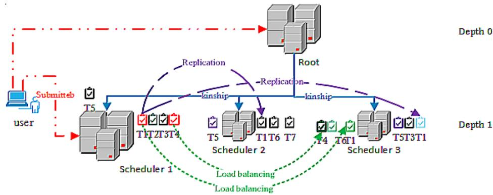
Figure 6. Inter-schedulers load balancing
