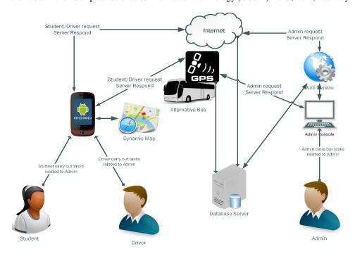
Figure.1 System Architecture
