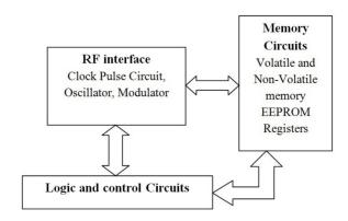
Figure 6. Components of RFID Architecture
