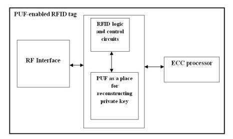
Figure 8. ECC based PUF-enabled RFID tag architecture
