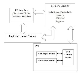
Figure 7. PUF-enabled RFID tag
