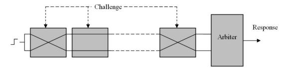
Figure 4. Arbiter PUF architecture
