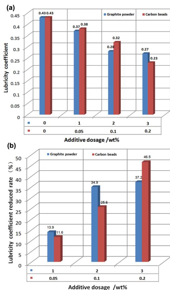
**Figure 4.** Lubricity coefficient (a) and lubricity coefficient reduced rate (b) of graphite powder and carbon beads in bentonite suspension (1 wt %) with different concentrations
