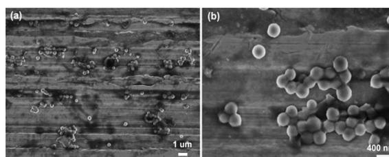
**Figure 7.** SEM images of the wear scar on steel disk after sliding under 1.0 N normal load for 40 min
