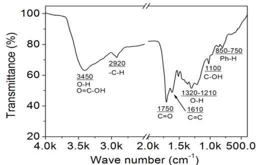
**Figure 2.** FT-IR spectra of as-prepared colloidal carbon beads
