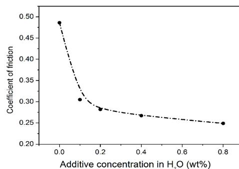
**Figure 6.** Coefficient of friction for various concentrations of carbon beads in water under 1.0 N normal load (Sliding speed : 5 cm/s, rotating diameter: 1 cm)
