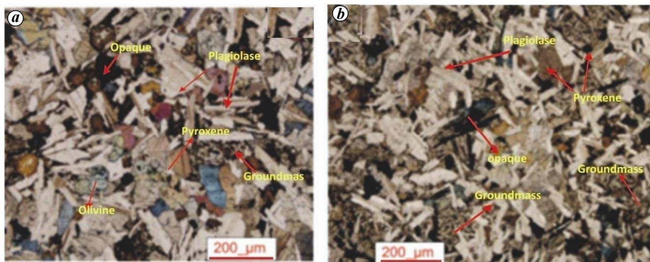
**Figure 2.** Photomicrographs of dyke samples: (a) Shahdol (RB-13) and (b) Chirimiri (RB-68B) dykes. The freshness of the plagioclase grains is noteworthy.
