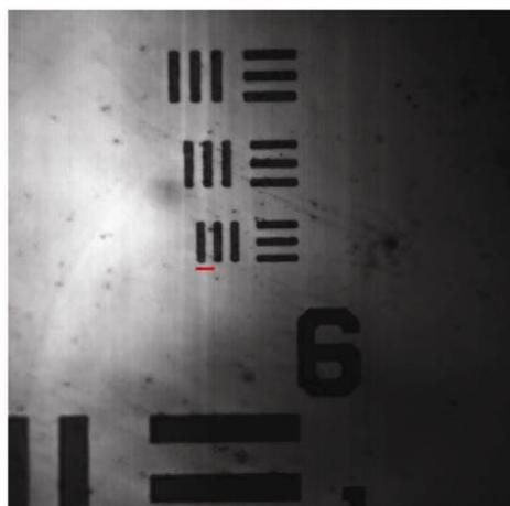
**Figure 3.** The 500 × 500 pixel image of 1951 USAF test target obtained by providing a saw-tooth waveform of 3V to the scan mirrors. There are 17 pixels between the smallest line pair (red line) corresponding to a specified distance of 1/228 mm. Thus, 500 pixels in the image correspond to 129 μm.
