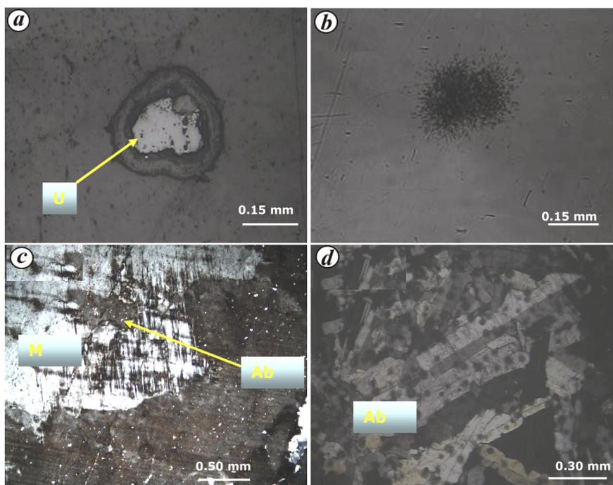
**Figure 4.** *a*, Uraninite (U) as inclusion in biotite from Nayagaon area. Note the reaction rim around uraninite grain. Reflected plane polarized light. *b*, High-density alpha tracks corresponding to uraninite of (*a*). *c*, Microcline (M) being replaced by albitite (Ab) in pegmatoid from Bichun area. Transmitted light under crossed nicols. *d*, Randomly oriented laths of albitite (Ab) in albitite of Ghasipura area transmitted light under crossed nicols.
