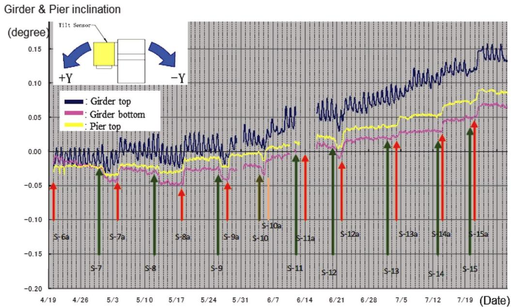
Figure 16. LEIS reading on transverse direction (XY) at P220.
