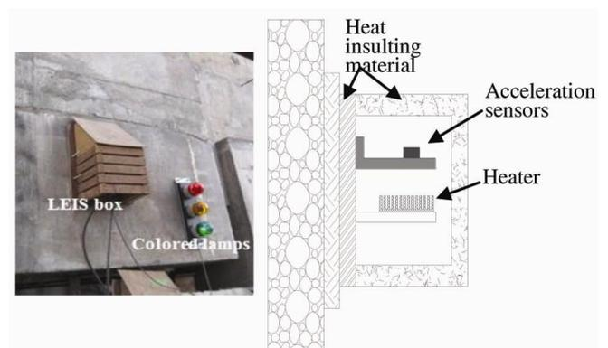
**Figure 4.** Light-emitting inclination sensor with coloured rotation lamps.
