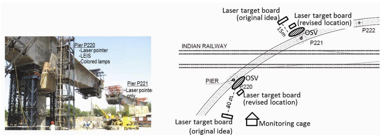
**Figure 5.** Arrangement of on-site visualization monitoring at site.
