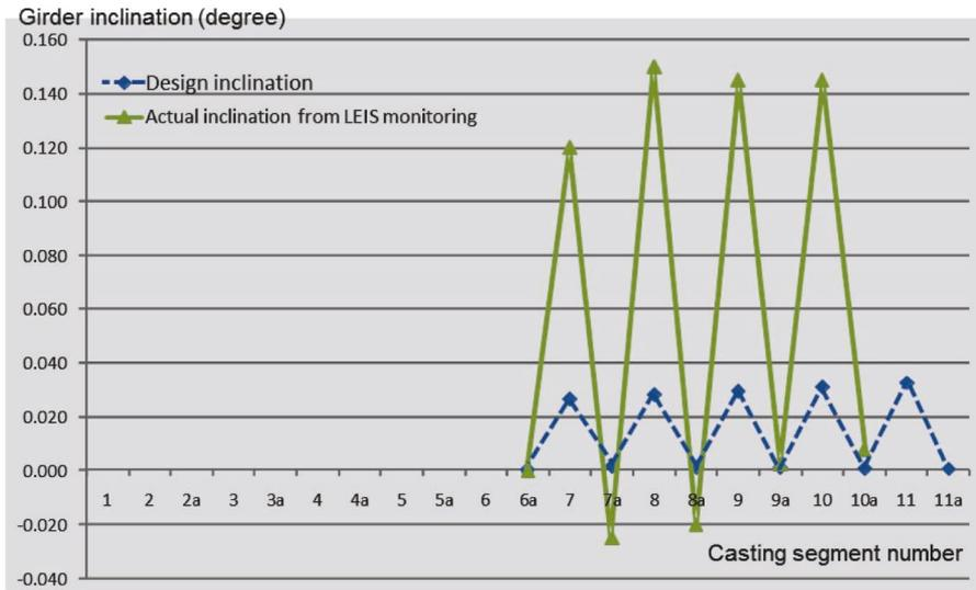
Figure 11. Bridge girder inclination on longitudinal direction ( $XZ$ ) at each stage at P220.
