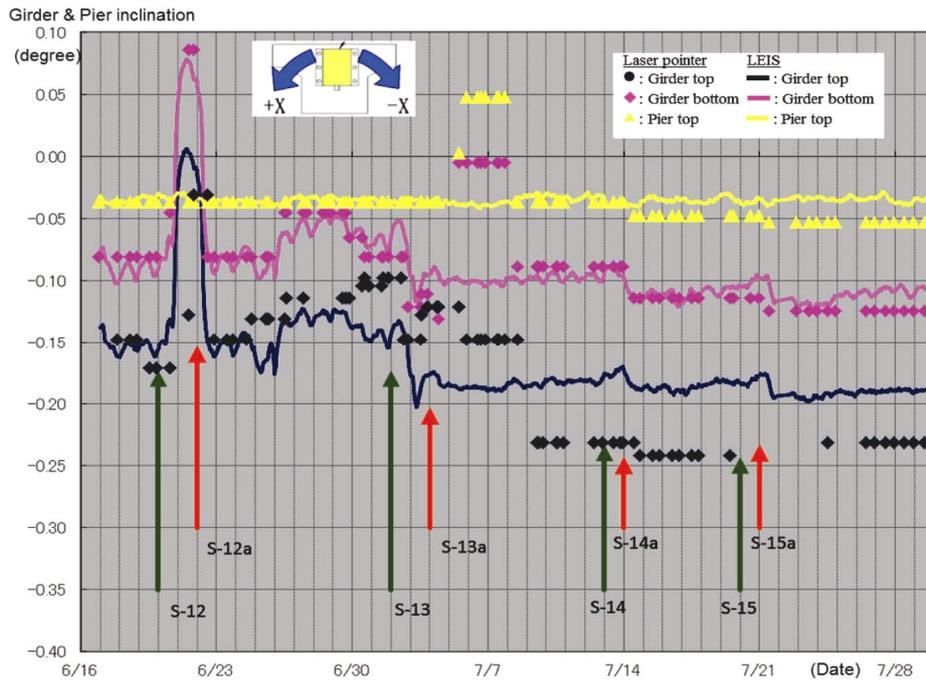
Figure 18. LEIS and laser pointer reading for longitudinal direction (XZ) at P220.
