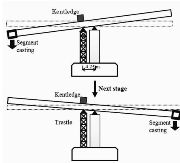
Figure 9. See-saw condition of bridge girder at each construction stage.
