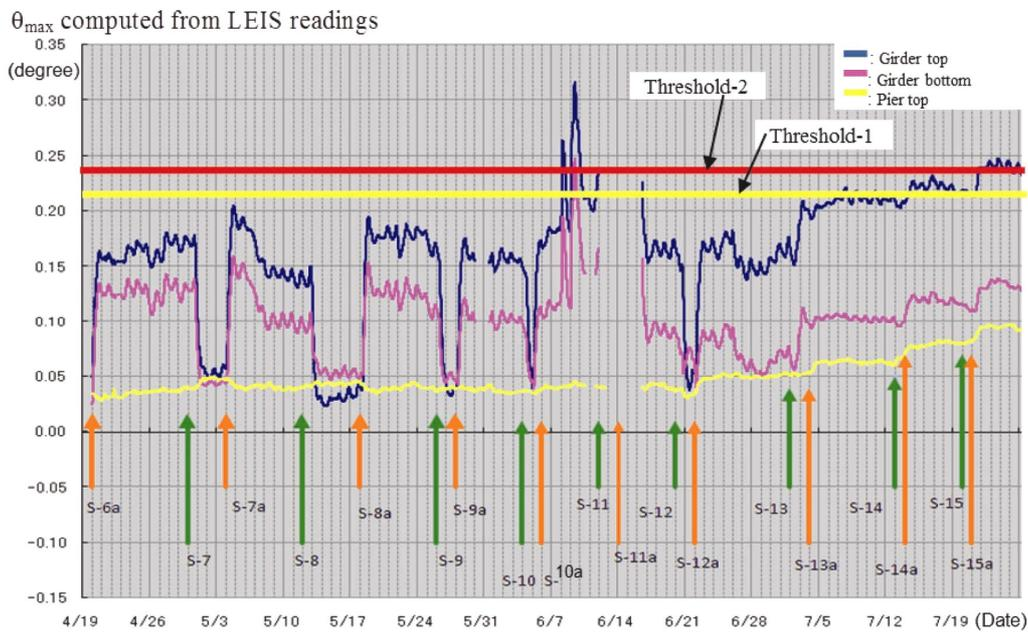
Figure 14. Maximum inclination (combined XZ and XY planes) by LEIS at P220.
