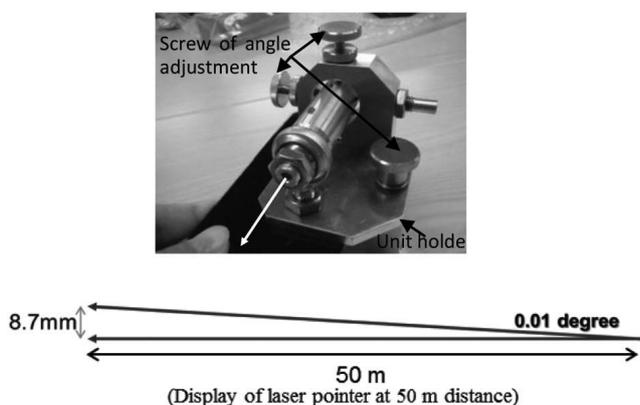
**Figure 3.** Laser pointer for inclination monitoring.
