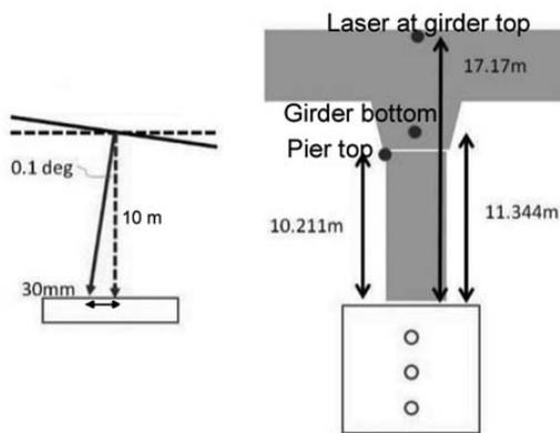
Figure 17. Concept of laser pointer reading.
