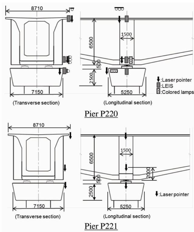
Figure 7. Detailed position of OSV devices at P220 and P221 (dimension in mm).
