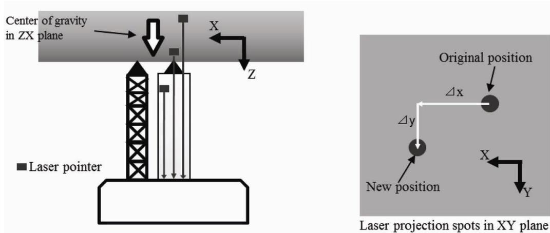
Figure 6. Schematic layout of laser pointers at P220 and P221.
