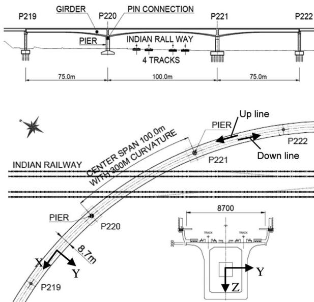
**Figure 2.** Plan and section of Okhla bridge.
