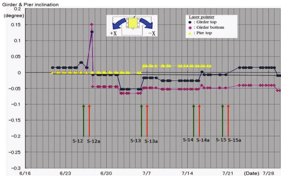
Figure 19. Laser pointer reading for longitudinal direction (XZ) at P221.
