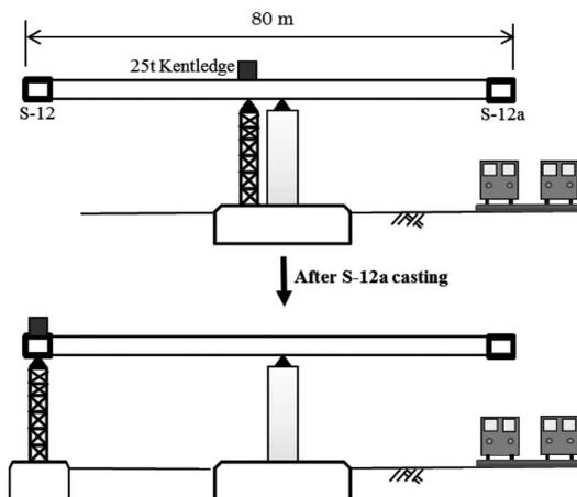
Figure 15. Shifting temporary support after segment casting S-12 and S-12a.
