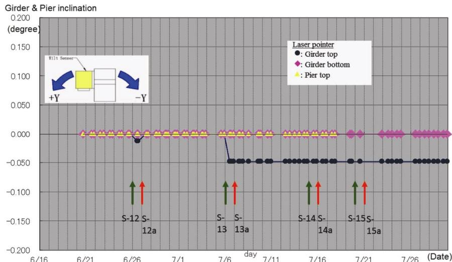
Figure 20. Laser pointer reading for transverse direction ( $XY$ ) at P221.
