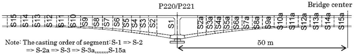
Figure 8. Order of segment casting by balanced cantilever construction methodology.
